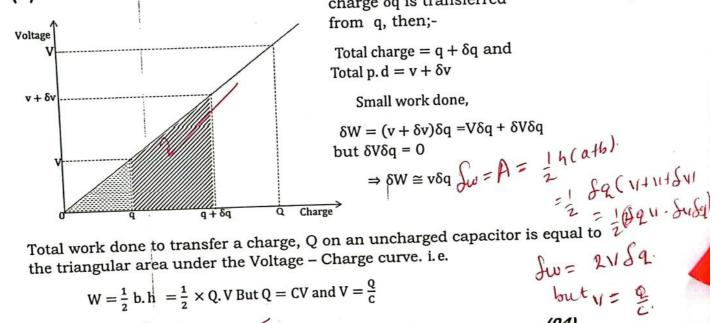
When a small amount of charge δq is transferred from q, then;-
