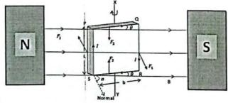
The forces  $F_1$  on the sides PS and QR are still given by  $F_1 = BILN$  because PS and QR are perpendicular to B.
